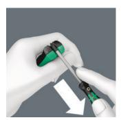
To demagnetise, move the tool along the negative side.
